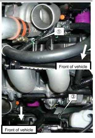
(13) Reinstall the factory intake manifold; then install Supercharger Bracket No.2 to the intake manifold using the factory bolt and Supercharger bracket No.1 with the following parts.
