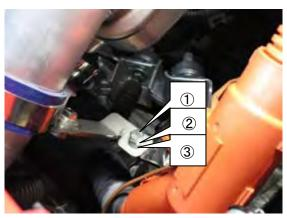
(21) Secure the Hose 8mm to ① using a tie wrap so the hose does not come in contact with other parts of the vehicle as shown the diagram on the right.
