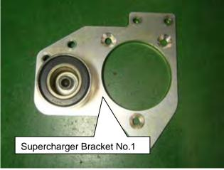
(5) Insert the Spacer M8 L=3.5 ② between the Supercharger Assy and the Supercharger Bracket. Install the Supercharger Assy to Supercharger Bracket No.1 using the Flat Head Bolt M8 L=35 ①.
