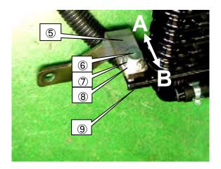
(11) Remove bolts ① and ②, and install the Oil Cooler Assy to the vehicle. XOnly for a JDM vehicle.
