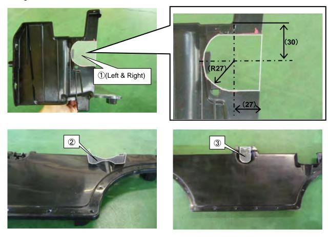
(28) Install the modified resin part of the factory front bumper air guide to the vehicle using the factory bolts and clips.
