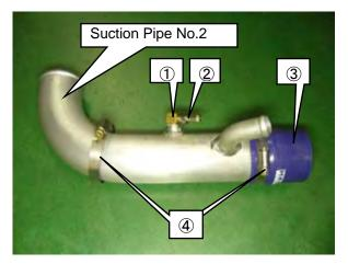
(33) Install the Restrictor ① to Suction Pipe No.2.
