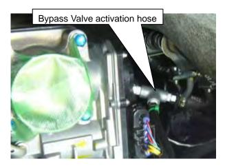
(25) Connect a 4mm rubber hose from the 3 way fitting to the Bypass Valve Assy using a Tie Wrap ①.
