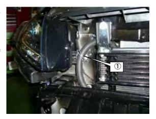
(15) Connect the 1250mm Hose 8mm ① to the Oil Tank using the 8mm Hose Clip ②.
