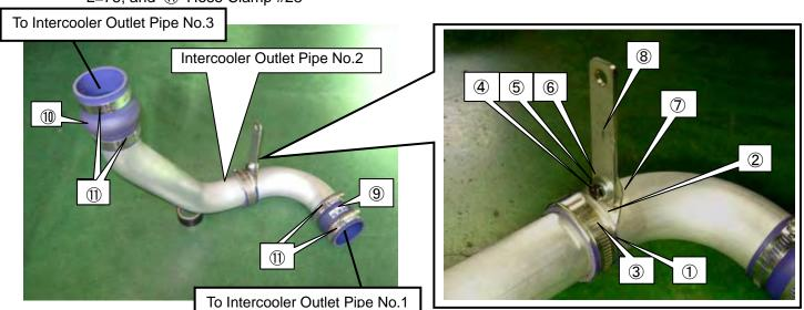
(15) Remove the bolt ① in the diagram below, and temporarily install Intercooler Outlet Pipe No.2 to the vehicle.
