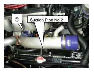
(35) Insert the Spacers M4 L=1.5 between the airflow sensor and Suction Pipe #3 and install the airflow sensor to Suction Pipe #3 using the factory bolts.
