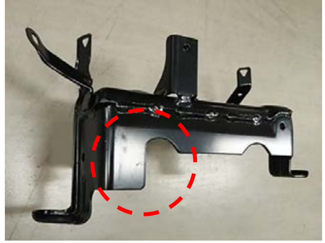
Injector Cover of Vehicle After 2012 (Modification is required.)
