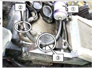
(19) Secure the Hose 8mm, Hose 10mm, and fluid filter to the vehicle.
