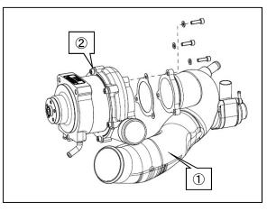
(5) Place the GT2-7040 on the S/C Bracket No.1 so as to the bracket comes in between the airflow sensor and supercharger.
