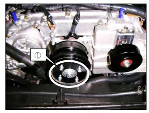
(2) Install ①Belt 7PK 1060. When the S/C pulley is installed to GT2-7040, use 7 ribs of the vehicle's rear side, and leave one rib of the vehicle's front side unused.
