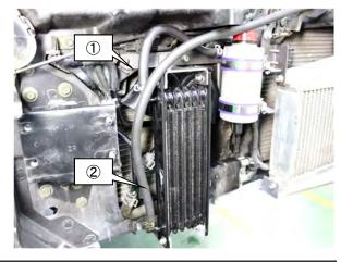
(16) Secure ①Hose 8mm to the power steering fluid pipe.
