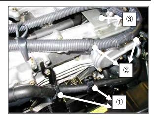
(10) Loosen the four M6 bolts on the ①Idler Pulley.
