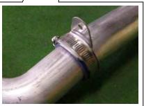
(11) Temporarily install the Intercooler Inlet Pipe No.1 assembly to the Supercharger Unit assembly.
