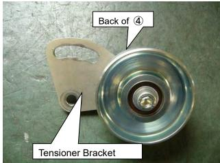
(8)Temporarily install the Supercharger Bracket No.2 to the engine using ①Cap Bolt M8 L=65, ②Washer M8, and ③Spacer M8 L=10.
