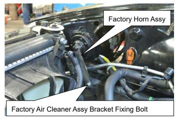
(14) Remove the vinyl tape from the factory horn coupler's end and install the factory horn coupler to the factory horn that was relocated.
