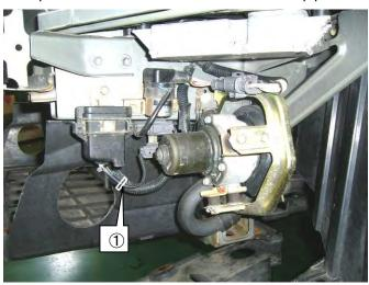
(27)Temporarily install the following parts to Intercooler Outlet Pipe No.1:
