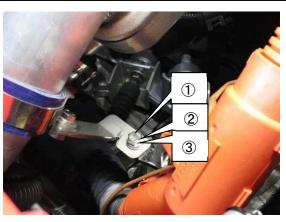
(20) Secure the Hose 8mm to ① using a tie wrap so the hose does not come in contact with other parts of the vehicle as shown the diagram on the right.
