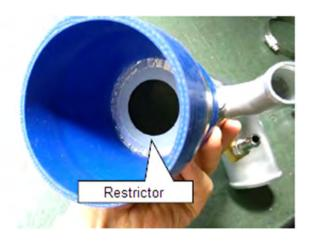
(34)Temporarily install the Suction Pipe No.2 Assy to the vehicle using the Hose Band #36 used in (33).
