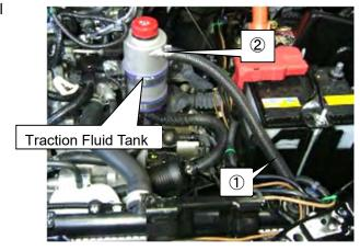
(16) Secure the Hose 8mm to ① using the Tie Wrap as shown in the diagram so the hose does not come in contact with other parts of the vehicle.
