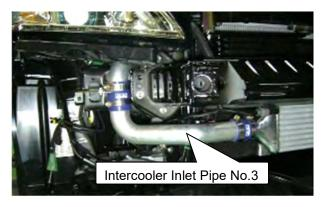
(11) Temporarily install Intercooler Inlet Pipe No.1 to the vehicle using ①Silicone Hose 50mm L=55 and ②Hose Band #28. After properly adjusting the positions of Intercooler Inlet Pipe No.1, 2 and 3, tighten all bolts and hose clamps temporarily installed.
