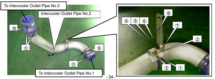
(14) Remove the bolt ① in the diagram below, and temporarily install Intercooler Outlet Pipe No.2 to the vehicle.
