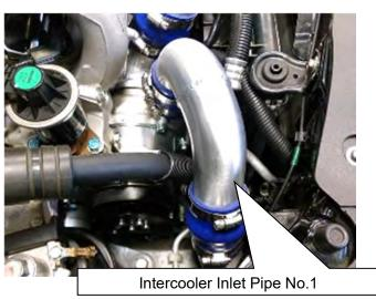
To Intercooler Inlet Pipe No.2
