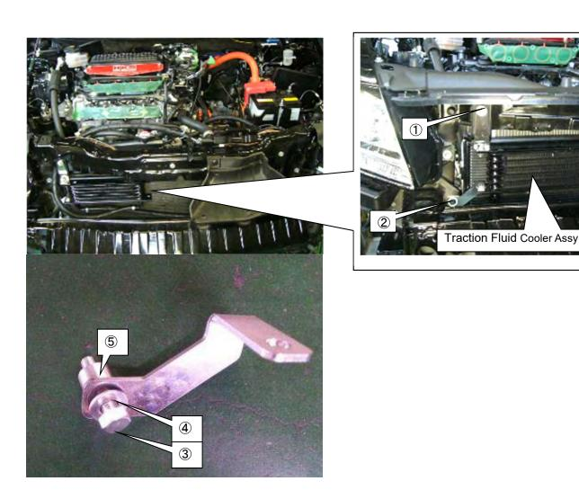
(13) Pull the 1000mm Hose 8mm ① and the 1250mm Hose 8mm ② from the both ends of the A/C condenser to the engine room.
