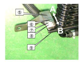
(11) Remove bolts ① and ②, and install the Traction Fluid Cooler Assy to the vehicle. XOnly for a JDM vehicle.
