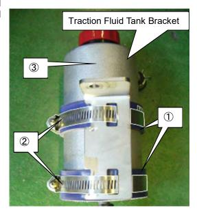
(6) Remove the rubber cap from the hose fitting on the lower part of the Traction Fluid Tank and connect the Hose 10mm ② using the Hose Clip 10mm ①.
