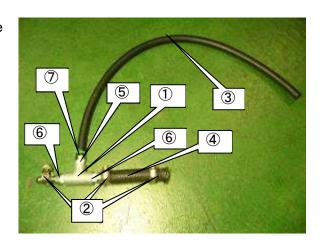
(23) Remove the factory vacuum hose, and install the 3 way fitting Assembly between the intake manifold and factory vacuum hose.
