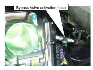
(24) Connect a 4mm rubber hose from the 3 way fitting to the Bypass Valve Assembly using ①Tie Wrap.
