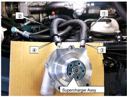
(8) Install the Supercharger Assembly to Supercharger Bracket No.1 using ① Flat Head Bolt M8 L=35.
