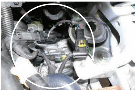
Connect the harness of BOOST CONTROLLER
