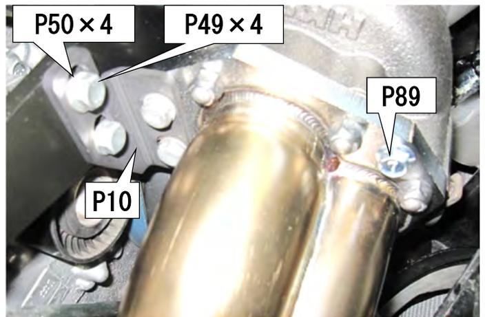
(6) Temporarily attach the front pipe side of the extension pipe to the joint pipe via the gasket. At this time, co-tighten the extension bracket attached in 5-(4).
