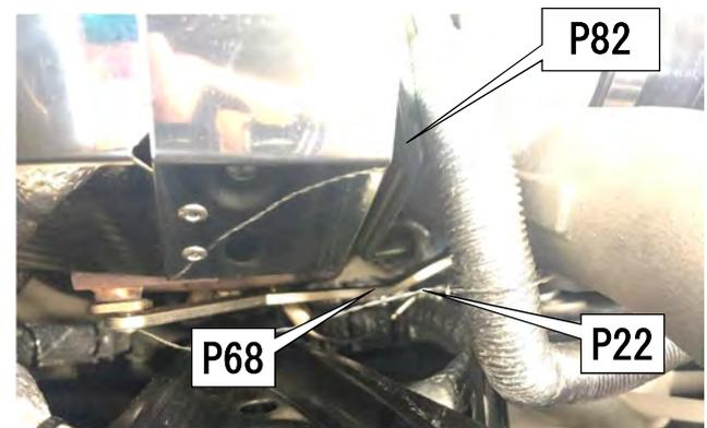
(6) Install the Oil Inlet Hose temporarily installed in the section 3 to the turbocharger.
