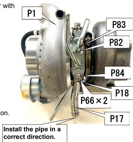
(2) Install the Stud Bolt M8 to the Turbocharger Assembly.
