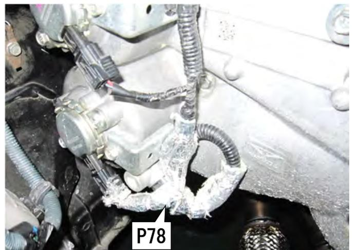
(3) Install the provided Insulator  $\phi 60$  to the Extension as shown in the photo on the right, and secure it with the provided Hose Band #40.
