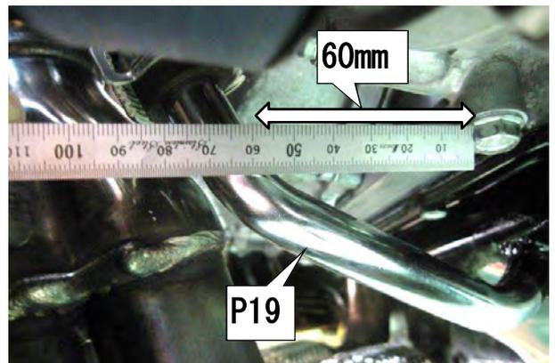
(14) Remove the oil pan. Weld the Oil Return Pipe to the oil pan.
