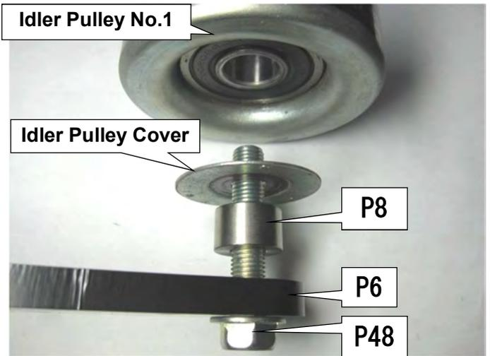
(5) Temporarily install the Flange Bolt M6 L10 as shown in the photo on the right.
