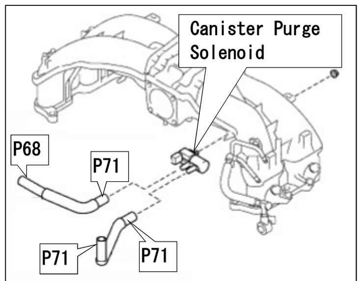
(21) Reinstall the canister purge solenoid. Place the throttle body and A/C compressor back in place.
