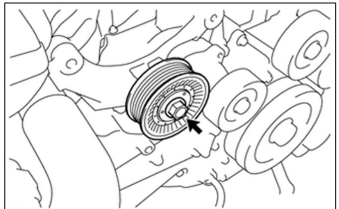
(4) Install the Turbocharger Bracket No.1, Stepped Spacer O.D.  $\phi$  20, Spacer O.D.  $\phi$  20, removed idler pulley cover, and idler pulley using the provided Flange Bolt M10 L50 7-mark.
