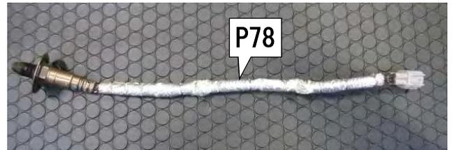
(2) Cut the provided Insulator Sheet to an appropriate size. Wrap the camshaft position sensor wire with the sheet and secure it with a wire.
