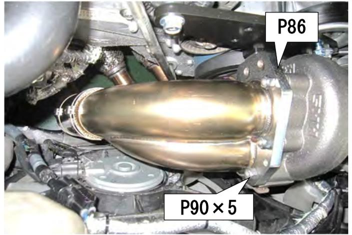
(6) Temporarily attach turbocharger bracket No. 3.
