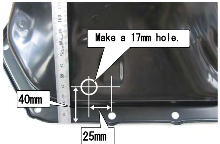
(12) Temporarily reinstall the oil pan, and temporarily install the Exhaust Manifold using the provided Gaskets.
