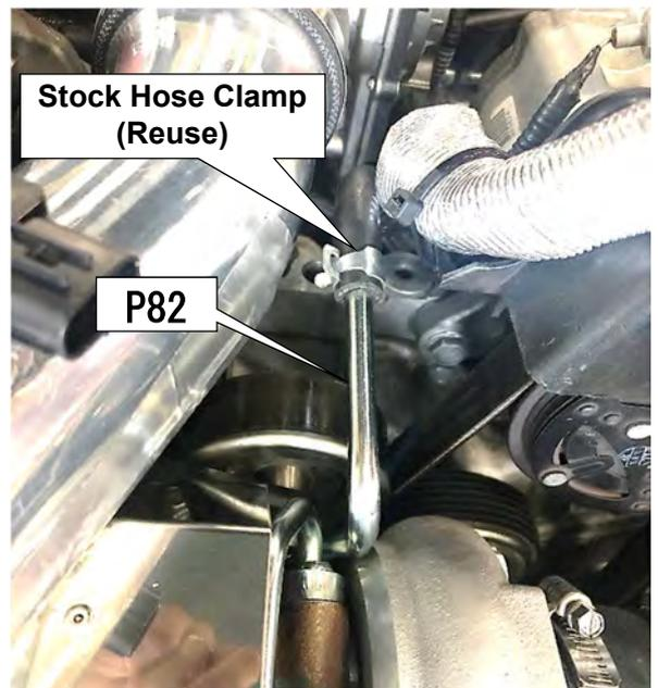
(3) Cut the provided Hose  $\phi 8$  to 1200mm in length. Connect the water line hose removed in (1). Secure the hose with the provided Hose Clamp Mark 130 as shown in the photo on the right.
