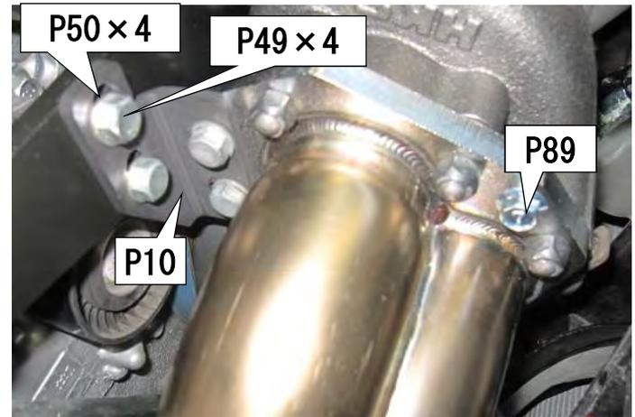
(7) Temporarily attach the front pipe side of the extension pipe to the joint pipe via the gasket. At this time, co-tighten the extension bracket attached in 5-(4).
