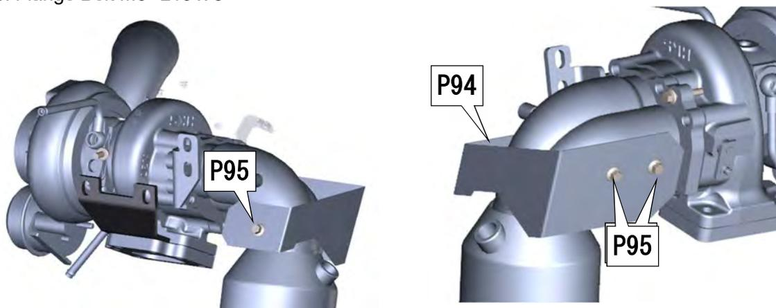
(8) Insert the Insulator into the Flange Bolt M6 L10 temporarily installed in section 4 and section 8 and tighten the bolts.
