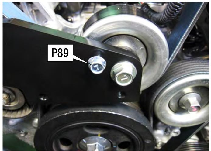
(6) Make sure the belt is placed on all pulleys. Remove the 3mm hexagonal wrench or a similar tool securing the belt. Make sure a proper tension is applied to the belt.
