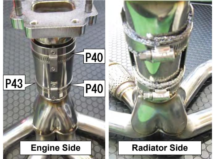
(3) Cut the Insulator Sheet to an appropriate size as shown in the photo on the right. Wrap the radiator hose with the Insulator Sheet and secure the sheet with a wire.
