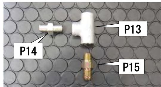
(3) Install the assembled fittings to the engine as shown in the photo on the right. Apply the ThreeBond TB1324 thinly to the PT thread.
