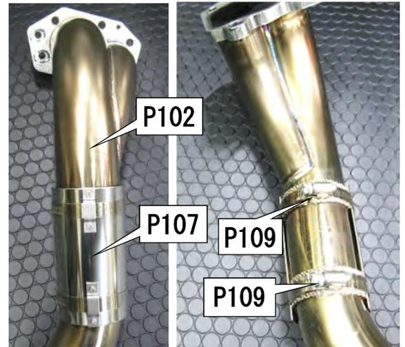
(4) Attach the A/F sensor and the O<sub>2</sub> sensor, attach insulators No. 1 and No. 2 to the catalyzer section of the extension pipe and fix them with a hose band.
