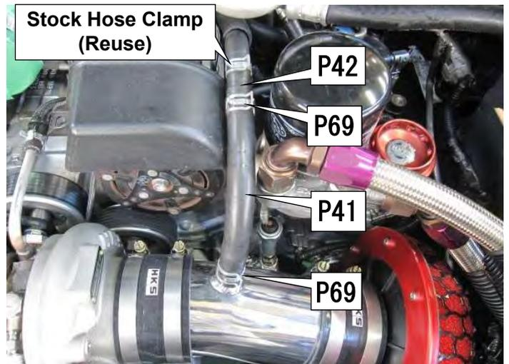
(5) Connect the Hose  $\phi 12$  from the Joint Pipe to the Suction Pipe. Secure the hose using the provided Hose Clamp Mark 180.
