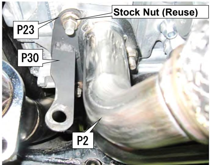
(5) Temporarily install the Turbocharger Bracket No.2 to the flange on the turbocharger side.
