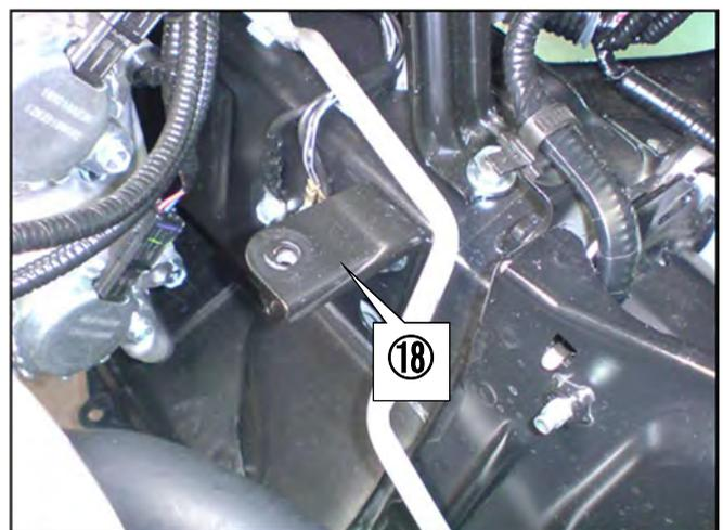
(20) Remove ⑱ fan shroud. (The removed shroud will be modified and reinstalled later.)
