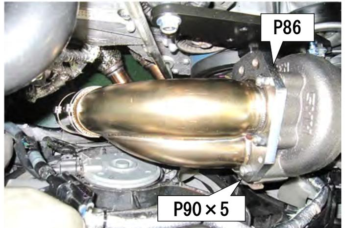
(5) Temporarily attach turbocharger bracket No. 3.
