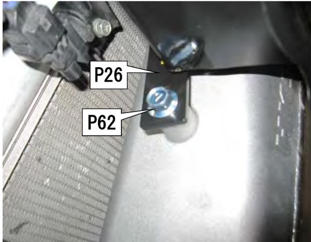
(5) Tighten all bolts completely after making sure the Intercooler does not come in contact with any other parts of the vehicle.
