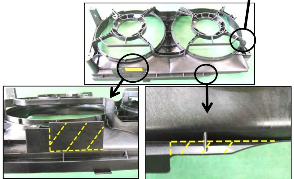
(8) Cut the Insulator Sheet 300 x 300 to an appropriate size and wrap the wire with a cut sheet.
