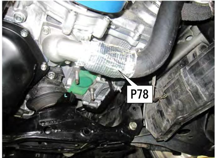
(4) Temporarily install the Exhaust Manifold using the provided Gasket and stock nut. The extension bracket is co-tightened to the flange.
