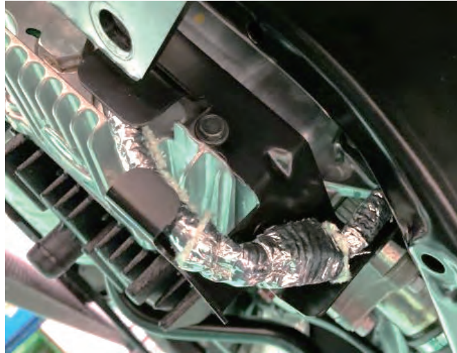
Fig.2 Diff Oil Temp Sensor Harness with Heat Insulation
