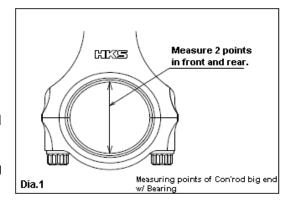
2-2. Measure the inner diameter of the big ends after installing the Bearings with the cylinder gauge as shown in diagram 1. Measure at least 2 points on the front and back. (Employ the smaller value to calculate the oil clearance.)
