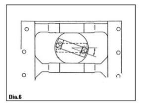
3.4 Install the Connecting Rod Caps as instructed above after applying clean engine oil. Each connecting rod cap should insert into the proper connecting rod in the correct direction.
