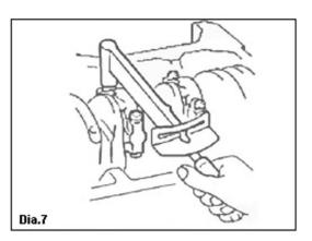
(3) Additionally, tighten 120 degrees. (Fastening angle) [NOTE]
