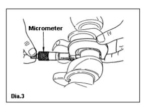
2-5. Calculate the oil clearance based on the inner diameter of the bearing measured in 2-1, 2-2, and the crank pin diameter measured in 2.5. Select the Bearings so the oil clearance should be within the designated clearance value according to the below formula.
