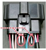
5. Divide the wires into [voltage group] and [pulse group] and attach corrugated tube, Y-manifold, and tube clip.
