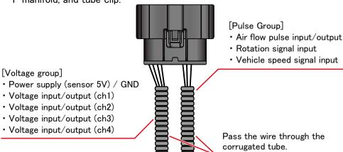
When branching corrugated tubes, use a Y-manifold.
