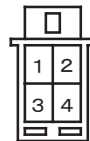
Figure of 4 pin connector of Universal Harness 1 & 2 viewed from the pin insertion side.
