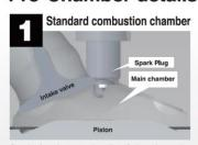
Spark plug tip protrudes directly into the main
