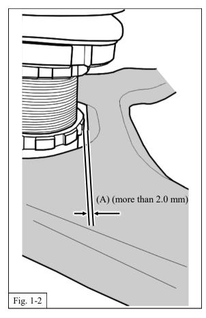
Check the clearance (A) of between the upper control arm and the suspension should be more than 2.0 mm at a 0 gravity state (Vehicle was jacked up) when installing the product. (Fig. 1-2)
