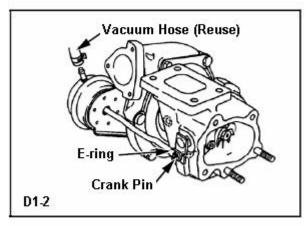
(6) Remove the actuator. (Diagram 1-3)
