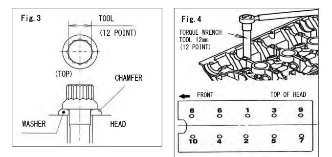
(4) Tighten the bolts with a torque wrench in the specified order in Fig. 4.
