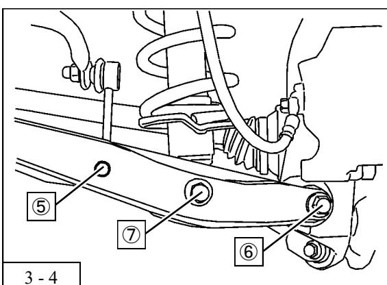
5. Remove the stabilizer link bolt and nut ⑤ .
