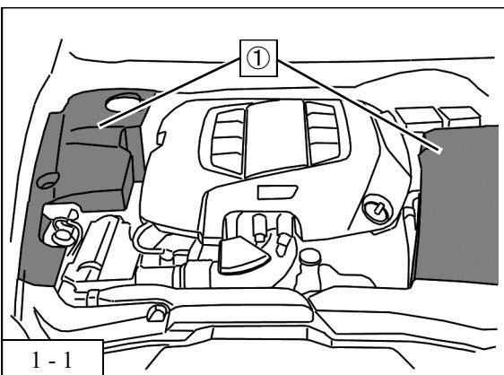
1. Remove the engine room side cover ① .
