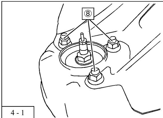
1. Install the provided rear suspension assy to the vehicle using the upper rear suspension assy installation nuts ⑧ .
