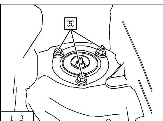
5. Remove the nuts from the upper front suspension assy ⑤ .
