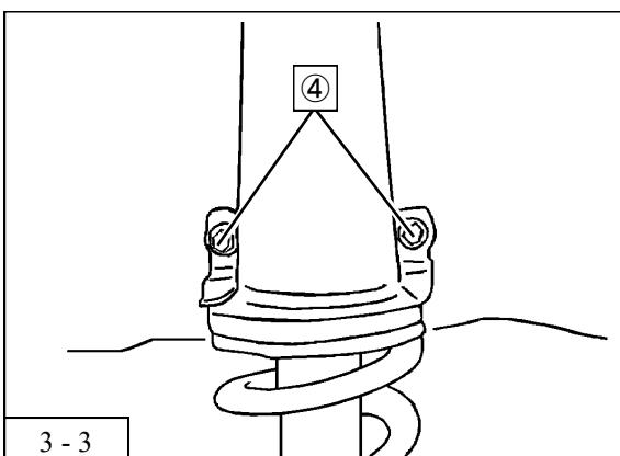
4. Remove the suspension support bolts ④ .
