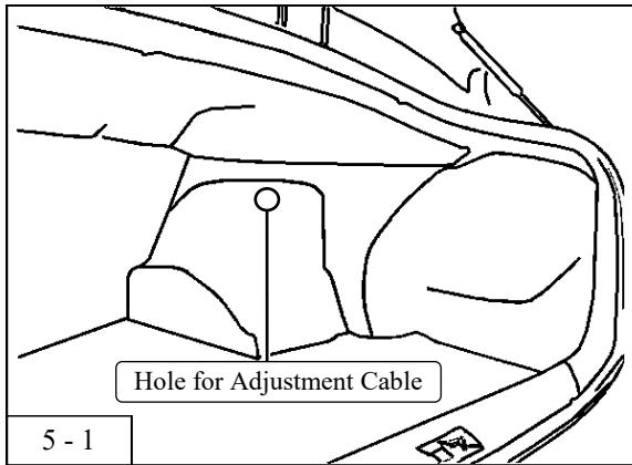
1. Make a hole for the adjustment cable in the trunk side trim.
