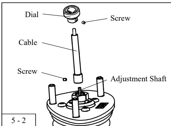
2. Remove the dial from the provided adjustment cable. Install the cable to the adjustment shaft on the tip of the rear suspension assy.
