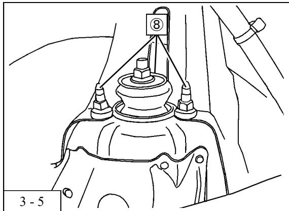
7. Remove the nuts from the upper rear suspension assy ⑧ .
