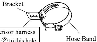
After installing the universal bracket, make sure tension is not applied to the ABS sensor harness when a steering wheel is turned and/or suspension is stroking.
