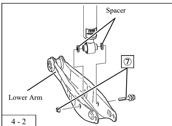
2. Install the provided spacers to both ends of the bush on the downside of the rear suspension assy, and install the bolt and nut for the lower rear suspension assy ⑦ . (Torque Specs: 110N·m)
