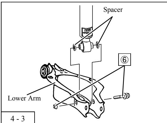
Install the provided spacers to the rear suspension assy when installing the rear suspension assy to the vehicle.
