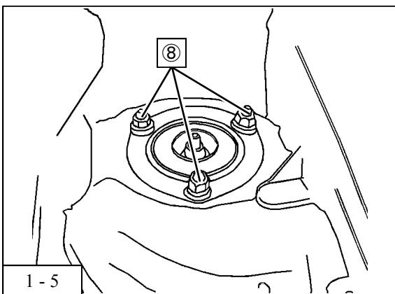
7. Remove the nuts from the upper front suspension assy ⑧ .
