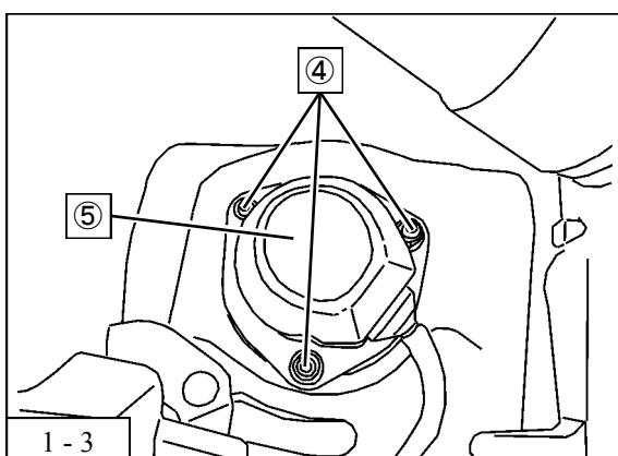
5. For a vehicle equipped with AVS, remove the following:
