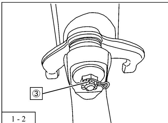
3. Remove the clip and upper arm joint nut ③ .
