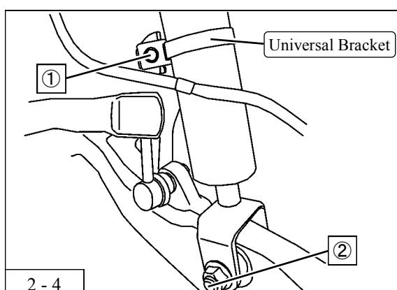
1. A universal bracket (a bracket & hose band) is included in this product to secure the ABS sensor harness. Secure the universal bracket to the front suspension assy where the measurement point can be the same position and distance as the factory suspension. (Diagram 2-1)
