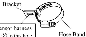
After installing the universal bracket, make sure tension is not applied to the ABS sensor harness when a steering wheel is turned and/or suspension is stroking.
