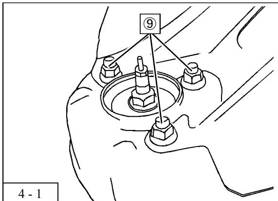
1. Install the provided rear shock absorber assy to the vehicle using the upper rear shock absorber installation nuts ⑨ .
