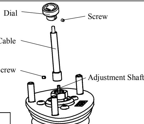
1. Install the provided long adjustment cable to the adjustment shaft on the tip of the rear suspension assy.
