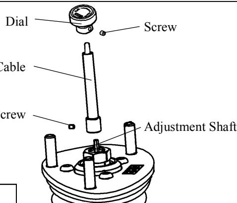
1. Install the provided short adjustment cable to the adjustment shaft on the tip of the rear suspension assy.
