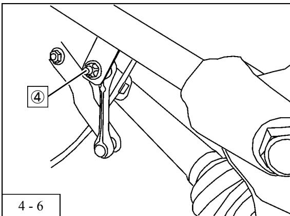
4. Install the provided spacers to both ends of the bush on the downside of the rear suspension, and install the bolt and nut for the lower rear suspension assy ⑥ . (Torque Specs: 110N·m)
