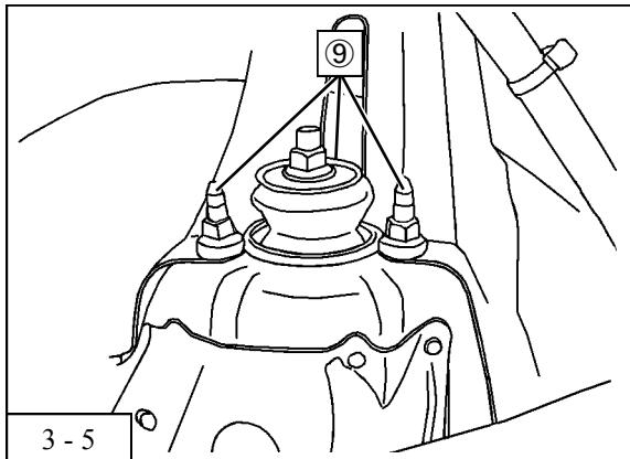
8. Remove the nuts from the upper rear shock absorber assy ⑨ .
