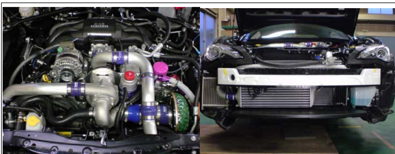
FA20 Engine with HKS GT Supercharger System
