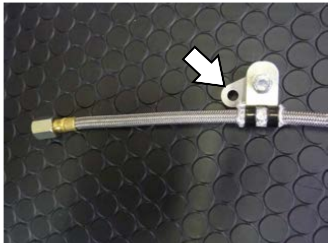
• VVT Oil Hose Bracket (t=2) • Hex Bolt M6 L=15 • Washer M6 • Flange Nut M6
