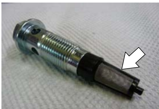
•Oil Filter attached to Banjo Bolt's Tip
