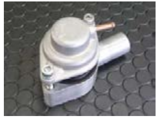
I3 : Blow-off Valve
