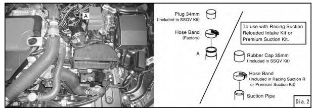
4. If the factory suction hose is used, install the joint pipe provided with this kit to "A" using the factory hose band. (Diagram Dia.2, Dia.3)
