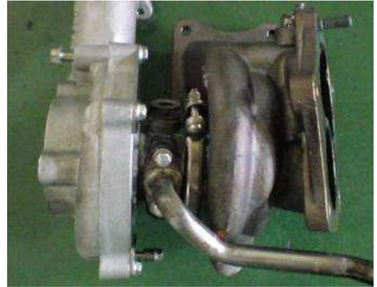
(12) Remove bolt ① from the Turbocharger Assembly. Install the factory turbocharger feed pipe to the Turbocharger Assembly using the following provided parts.
