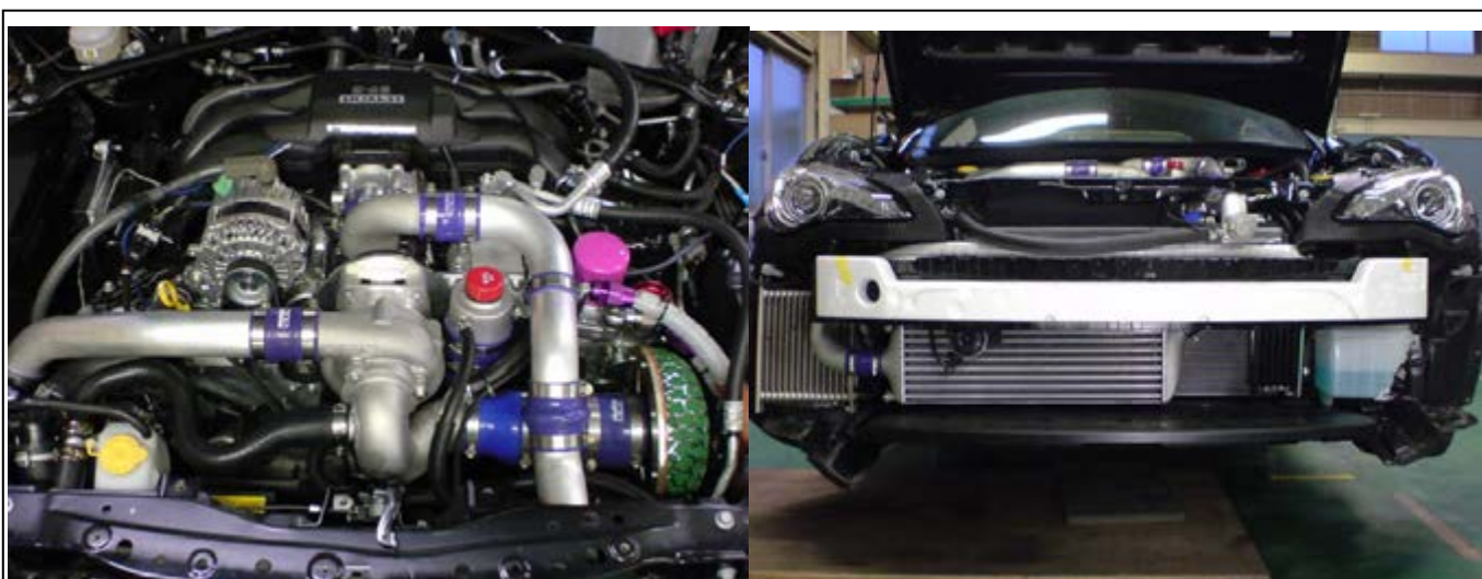
FA20 Engine with HKS GT Supercharger System
