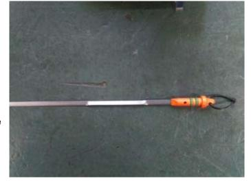
(4) Reinstall the modified factory engine oil level gauge back to the vehicle.
