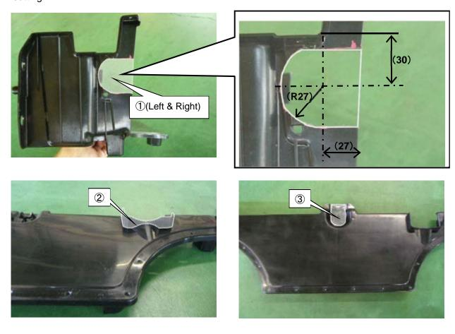
(27) Install the modified resin part of the factory front bumper air guide to the vehicle using the factory bolts and clips.
