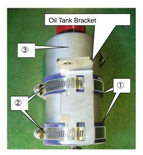
(6) Remove the rubber cap from the hose fitting on the lower part of the Oil Tank and connect the Hose 10mm② using the Hose Clip 10mm①.
