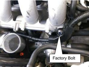
(14) Secure the Traction Oil Hose 8mm and 10mm with Tie Wraps at ①-③ in the diagrams on the right and below so the hoses do not come in contact with any other parts of the vehicle.
