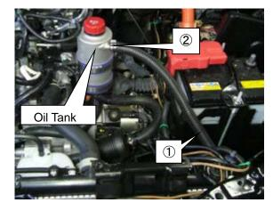
(16) Secure the Hose 8mm to ① using the Tie Wrap as shown in the diagram so the hose does not come in contact with other parts of the vehicle.
