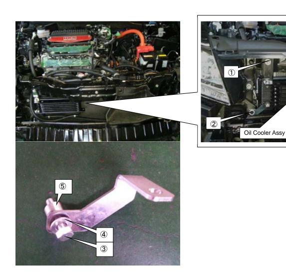
(13) Pull the 1000mm Hose 8mm ① and the 1250mm Hose 8mm ② from the both ends of the A/C condenser to the engine room.
