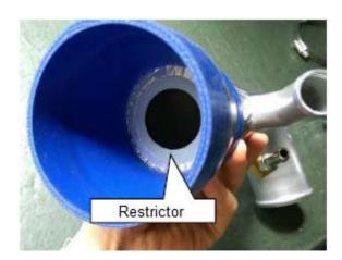
(34) Temporarily install the Suction Pipe No.2 Assy to the vehicle using the Hose Clamp #38 used in (33).
