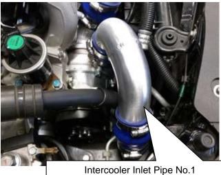
To Intercooler Inlet Pipe No.2
