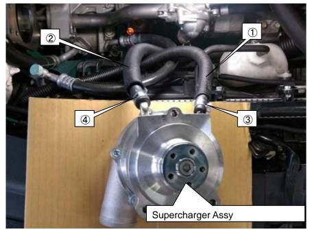
(8) Install the Supercharger Assy to Supercharger Bracket No.1 using ① Flat Head Bolt M8 L=35.
