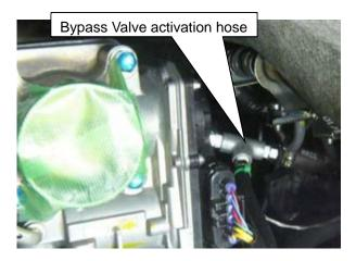
(24) Connect a 4mm rubber hose from the 3 way fitting to the Bypass Valve Assy using ①Tie Wrap.
