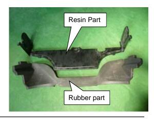
(26) Cut off ① on both sides of the resin part and ②, and the shaded portion ③.
