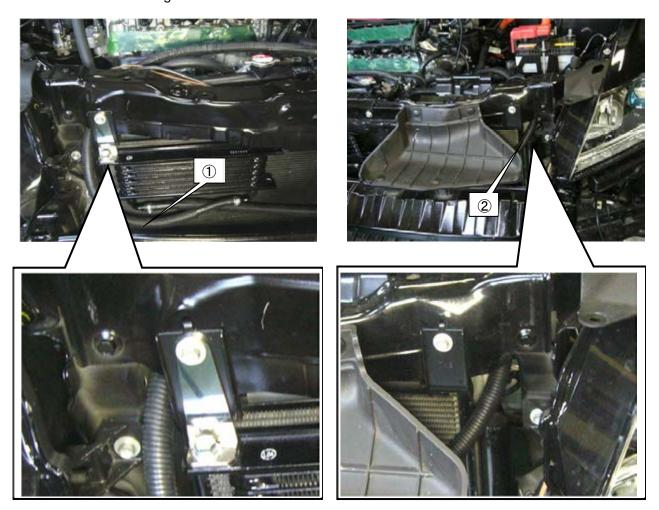
(14) Secure the Hose 8mm to ① using Tie Wraps as shown in the diagram so the hose does not come in contact with other parts of the vehicle.
