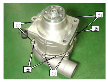
(6) Rotate the Supercharger unit and ③compressor Housing, and adjust the angle of the Supercharger Assy and compressor housing until there is 12mm gap between ④ the center line of the Supercharger Assy plate's both ends and ⑤ the center line of the compressor housing fixing bolt as shown in the diagram below. Retighten ①compressor housing fixing bolt and ②compressor housing fixing plate.
