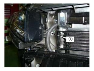
(15) Connect the 1250mm Hose 8mm ① to the Oil Tank using the 8mm Hose Clip ②.
