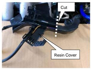
(13) After cut off the resin-made cover, cover the knock sensor harness and oil pressure sensor harness with the provided ① Corrugated Tube for Sensor Wiring. Secure the harnesses using the factory bolt as shown in the diagram below.
