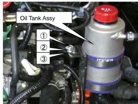
(8) Install the Elbow Fittings to the Oil Cooler ①.
