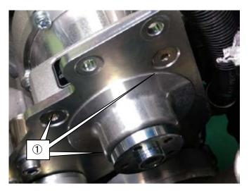
(9) Install the Supercharger Pulley to Supercharger Assy using ①Cap Bolt M6 L=18.
