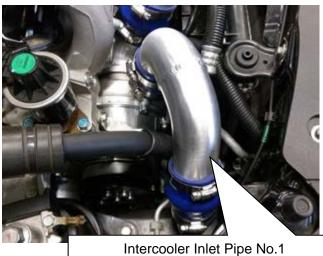
To Intercooler Inlet Pipe No.2
