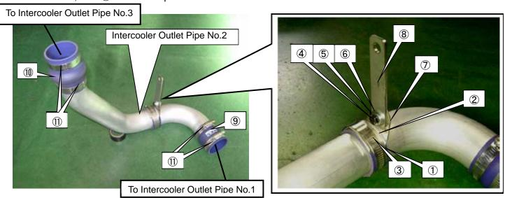
(14) Remove the bolt ① in the diagram below, and temporarily install Intercooler Outlet Pipe No.2 to the vehicle.
