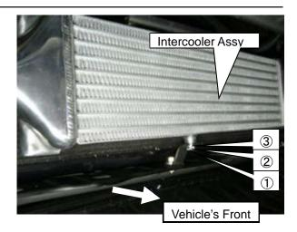
(7) Secure the Hose 8mm to ① in the diagram using tie wraps so the hose does not come in contact with any other parts of the vehicle.
