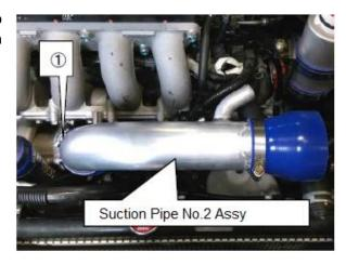
(35) Insert ①Spacer M4 L=1.5 between the airflow sensor removed from the factory air cleaner and Suction Adapter. Install the airflow sensor to the Suction Adapter using ②Button Bolt M4 L=12.
