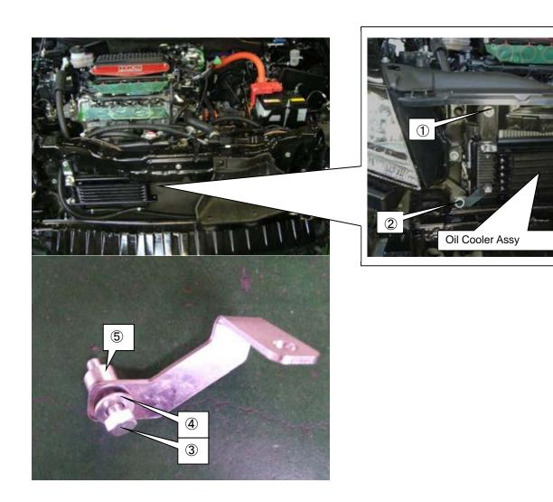
(13) Pull the 1000mm Hose 8mm ① and the 1250mm Hose 8mm ② from the both ends of the A/C condenser to the engine room.
