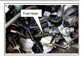
(14) Install the Fuel Hose assembled in (4) to the position where the stock fuel feed tube was removed from. Install the covers.
