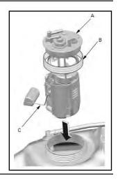
(14) Align the mark "B" on the fuel pump module with the mark "C" on the fuel tank. Press the fuel pump module in the vertical direction until it adheres to the packing.
