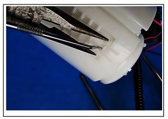
(2) Remove the fuel pump from the fuel sender unit.
