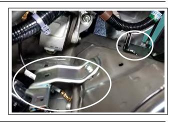
(7) Disconnect the fuel feed tube "A" from "B" and "C". Remove the clamp "F".
