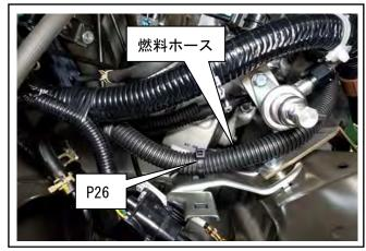
(16) Secure the harnesses cut off in 1.(5) indicated by circles using clamps.
