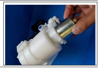
(5) Remove the pressure regulator from the fuel sender unit.
