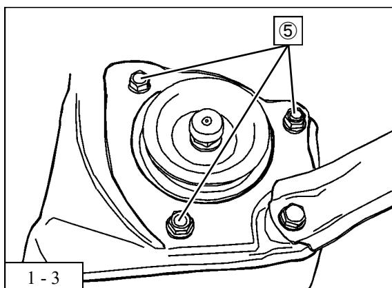
3. Remove the nuts from the upper front suspension assy ⑤ .
