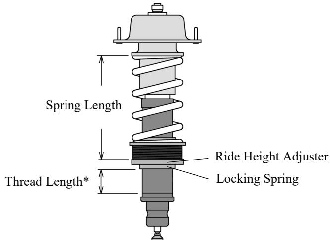
\*Thread length is the length between the bottom of the Locking Spring to the bottom of the cylinder screw.
