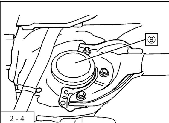
5. Install the strut rod cap ⑧ . (Torque Specs: 50N·m)
