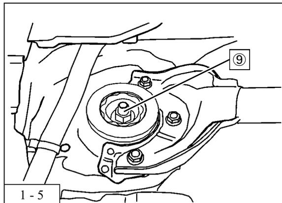
6. Remove the nut from the upper front suspension assy ⑨ .
