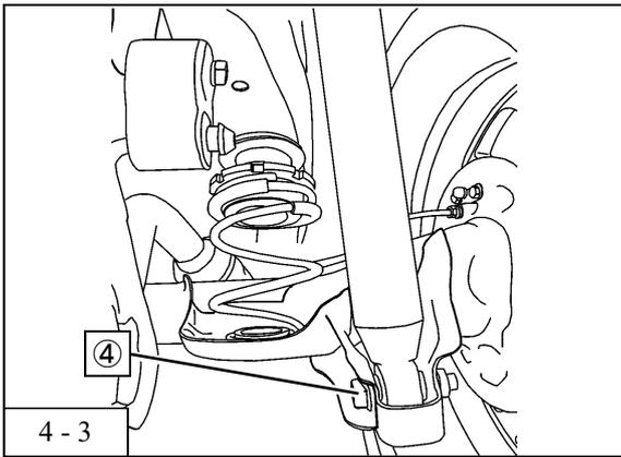
5. Lower the vehicle body down, completely tighten the lower rear shock absorber assy installation bolt ④.
