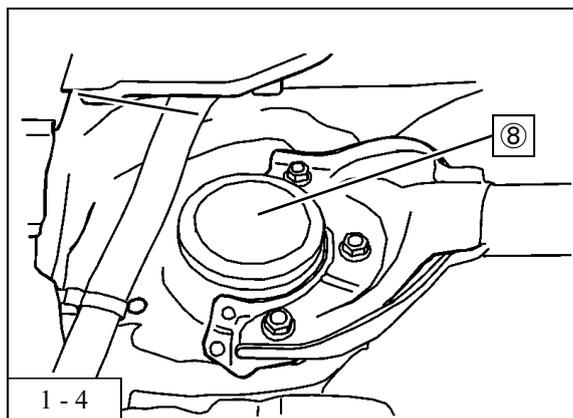
5. Remove the strut rod cap ⑧ .
