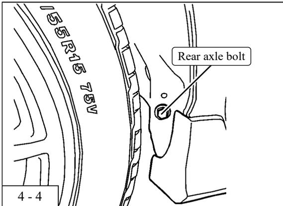
6. Loosen the rear axle bolt once, and retighten it.
