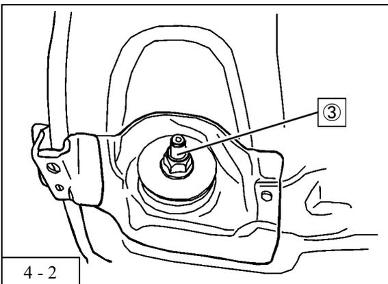
3. Install the factory parts to the provided rear shock absorber assy referring to “Suspension Components” on page 6.
