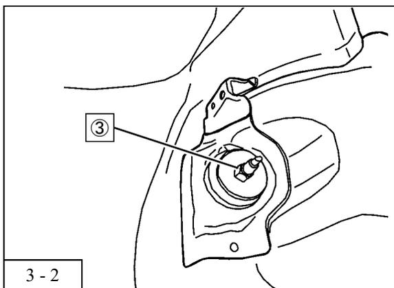
3. Remove the nut from the upper rear shock absorber assy ③ .
