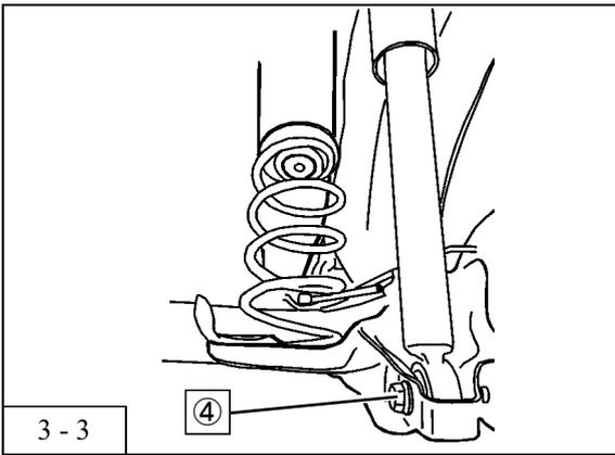
4. Remove the nut from the lower rear shock absorber assy ④ .
