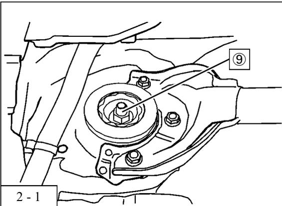
1. Install the upper front suspension assy installation nut ⑨ .
