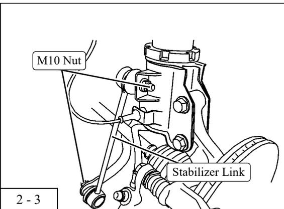
3. Install the provided stabilizer link using the provided M10 nuts.
