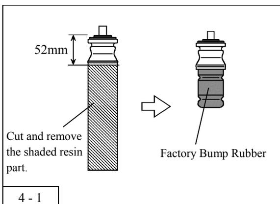
1. The factory upper mount is required to install the provided rear shock absorber assy. Remove the dust boots from the rear suspension support assy as follows:
