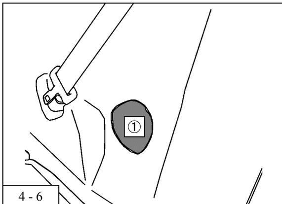
8. Reinstall the side hole cover ① to the vehicle.
