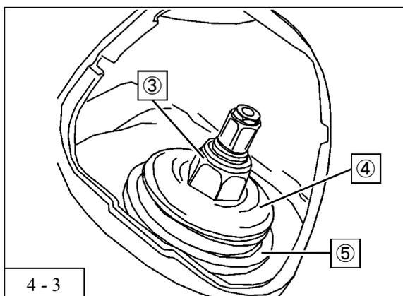
4. Install the following to the vehicle while supporting the axle beam's bottom with the jack:
