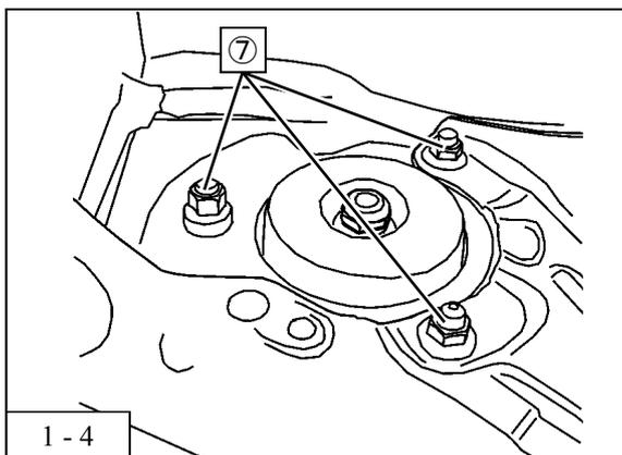
5. Remove the nuts from the upper front suspension assy ⑦ .
