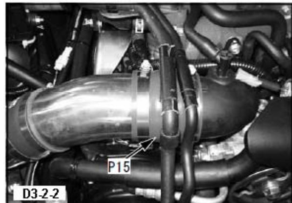
(4) Install the hose clamps removed in 3-2.(1) to the positions indicated in Diagram 3-2-3.
