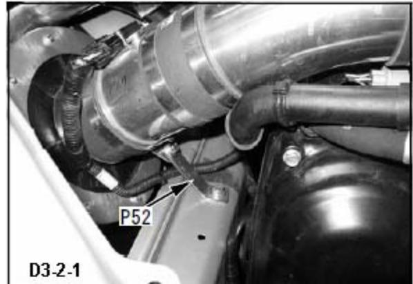
(3) Use the provided Purple Silicone Hose 75mm to install the air intake pipe instead of the joint hose 75mm instructed in 2.(3) of the Racing Suction Intake Kit instructions. (Diagram 3-2-2)
