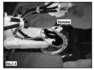
(5) Disassemble the fuel pump assembly, and remove the factory fuel pumps. (Diagram 2-5, 2-6) The removed case, wires, and filters will be reused later.
