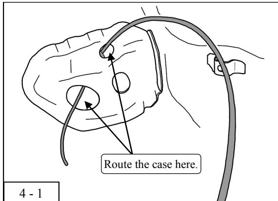
1. Route the adjustment cable outer case through the hole in the vehicle body.
