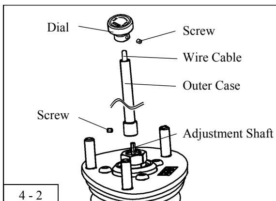
2. Adjust the screw's position to the flat section of the adjustment shaft's side. Use the provided Allen wrench to tighten the screw. (Diagram 4-2)
