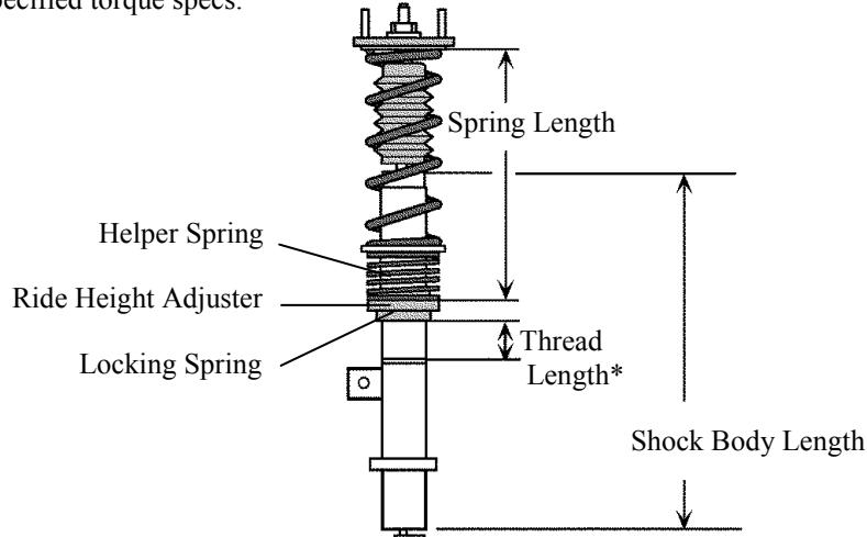
\*Thread length is the length between the bottom of the Locking Spring to the bottom of the cylinder screw.
