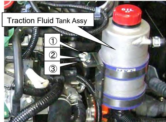
(8) Install the Elbow Fittings to the Traction Fluid Cooler ①.
