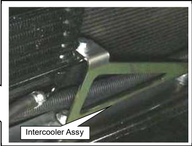
(6) After properly adjusting the position of the Intercooler Assy with enough clearance from surrounding parts, and install the Intercooler Assy to the vehicle using the following parts.
