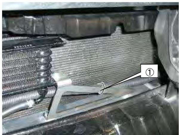
• Installation of Intercooler Inlet Pipe
