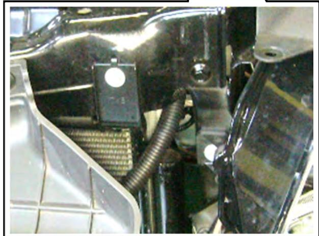
(14) Secure the Hose 8mm to ① using Tie Wraps as shown in the diagram so the hose does not come in contact with other parts of the vehicle.
