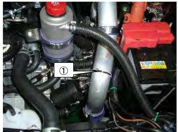
(21) Cut the Oil Resistant Hose 10mm to 80mm and 620mm in length. Cut the Hose 4mm to 450mm in length.
