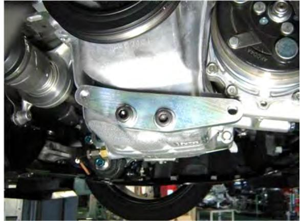
(16) Install the Pulley 60mm to Tensioner Bracket No.1 using the following parts.
