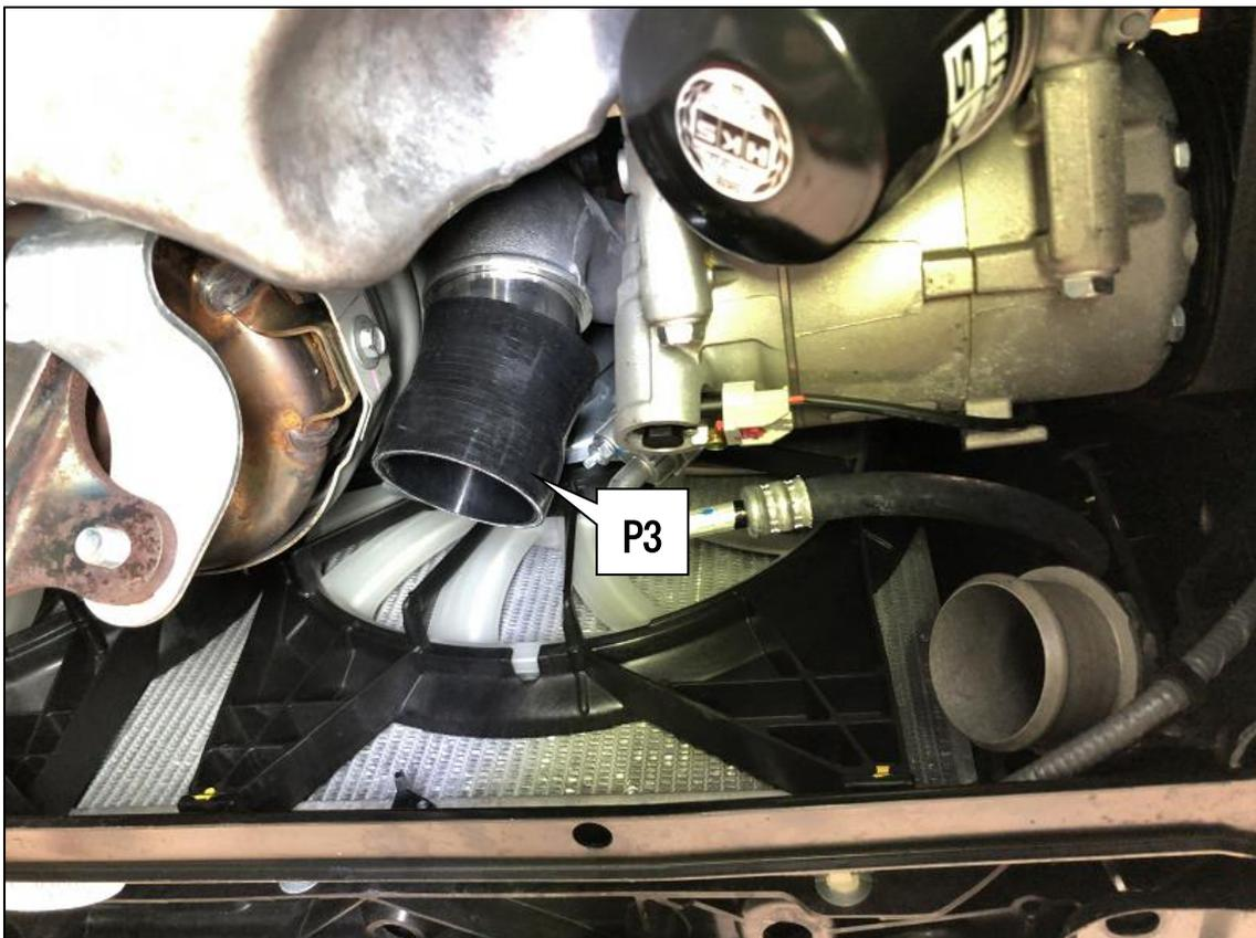
(3) Install the Intercooler Inlet Pipe to the turbocharger and intercooler.
