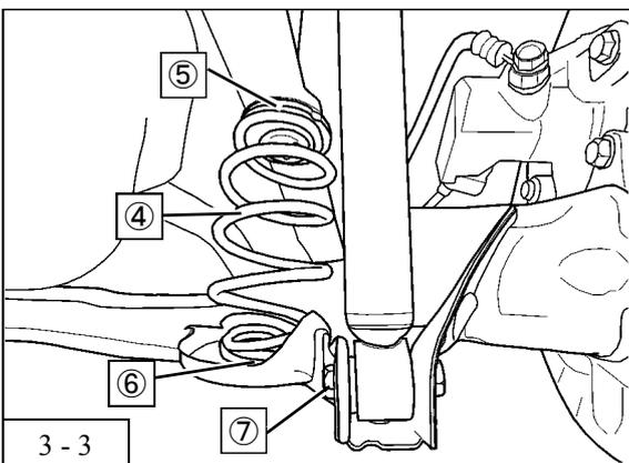
4. After loosening the lower installation bolt of the rear shock absorber assy installation bolt (7), remove the jack from the axle
