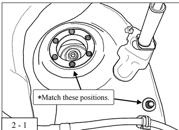
1. While positioning the upper mount assy positioning bolt's to a proper direction, align the upper mount assy's step to the hole in the body and press it down.
