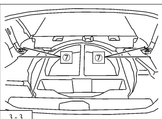
4. Remove the nuts from the upper rear suspension assy ⑦ .
