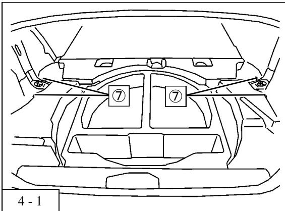
1. Install the provided rear suspension assy to the vehicle using the upper rear suspension assy installation nuts (7).
