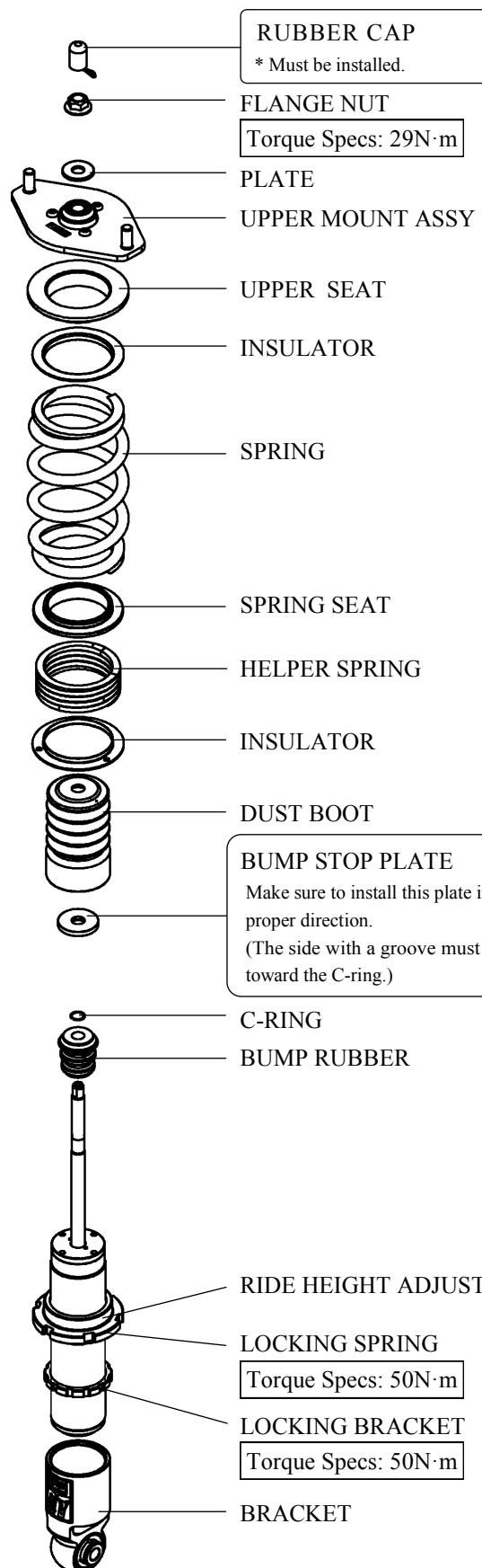
\* Torque value when tightened with the provided Spanner Wrench (Slotted).
