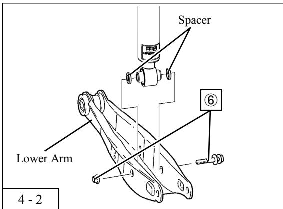
2. Install the provided spacers to both ends of the bush on the downside of the rear suspension assy, and install the nut for the lower rear suspension assy (6).
