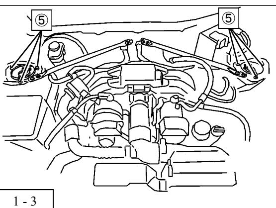
4. Remove the nuts from the upper front suspension assy ⑤ .
