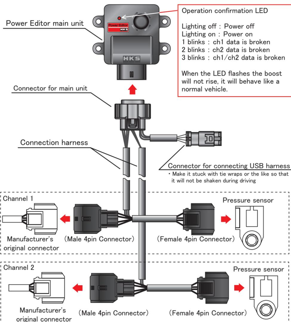
4. Disconnect Manufacturer's original connector from Pressure sensor, and wire the connection harness of Power Editor.
