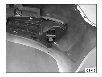
(6) Remove 3 bolts and 1 nut from both sides to remove the bumper reinforcement. Diagram 3-6 shows only one side; remove bolts and nut from the opposite side as well.
