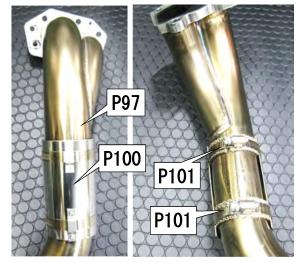
(4) Fit the extension pipe assembled in (3) with the gasket to the turbine and temporarily attach it with the locknut.
