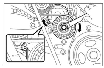
(2) Remove the idler pulley No.1 as shown in the diagram on the right.
