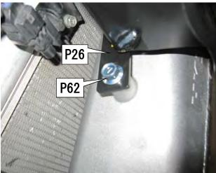
(5) Tighten all bolts completely after making sure the Intercooler does not come in contact with any other parts of the vehicle.
