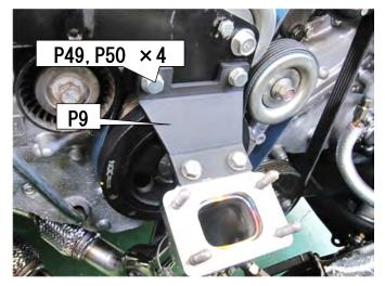
(6) Determine the installation position of the Exhaust Manifold; then tighten the Turbocharger Bracket No.2 completely.
