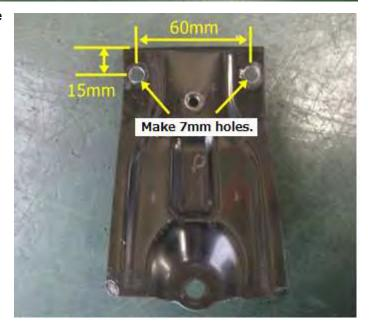
(5) Cut the radiator support as shown in the photo on the right.
