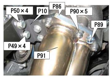
Flange bolt M6 L10 is that for installing an insulator later work.
