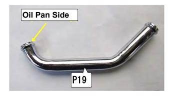
Make sure the clearance between the exhaust manifold and Oil Return Pipe is at least 15mm.
