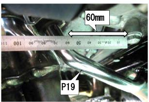
(14) Remove the oil pan. Weld the Oil Return Pipe to the oil pan.
