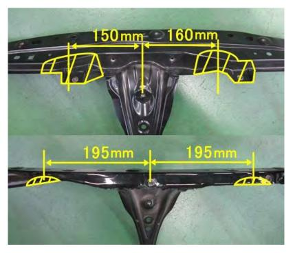
(6) Cut the fan shroud as shown in the photos on the right side.
