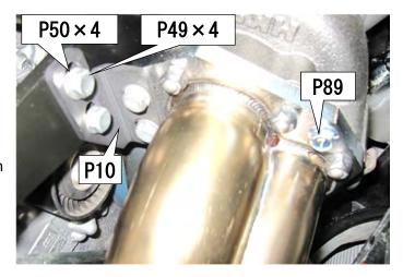
(6) Temporarily attach the front pipe side of the extension pipe to the joint pipe via the gasket. At this time, co-tighten the extension bracket attached in 5-(4).
