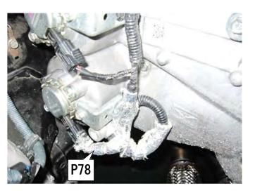
(3) Install the provided Insulator  $\phi$ 60 to the Extension as shown in the photo one the right, and secure it with the provided Hose Band #40.
