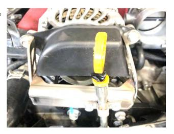
(12) Check that the O-ring on the oil level gauge pipe has not come loose from the engine and install the level gauge.
