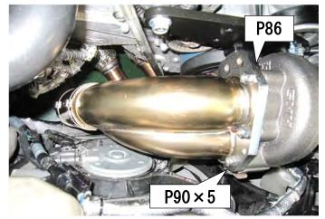
(5) Temporarily attach turbocharger bracket No. 3.
