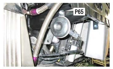
(5) Relocate the sponge on the hood support rod to the position shown in the photo on the right.
