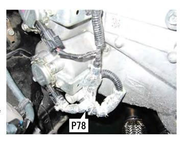
(3)Install the provided Insulator φ60 to the Extension as shown in the photo one the right, and secure it with the provided Hose Band #40.
