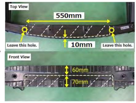
(2) Install the Flange Bolt M6 L15 from the back of the right side hole in the reinforcement.
