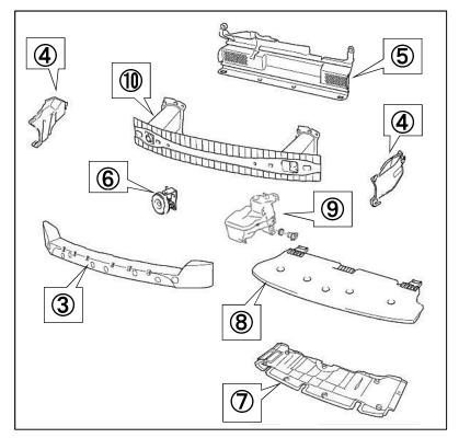
(12) Shift ⑨washer tank and remover ⑩reinforcement. (The removed reinforcement will be modified and reinstalled later.)
