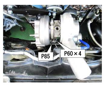
(4) Connect the Hose from the Oil Return Pipe to the Oil Outlet Pipe from the Turbocharger Assembly. Secure the hose with the provided Hose Clamp Mark 230.
