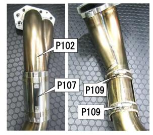
(4) Attach the A/F sensor and the O₂ sensor, attach insulators No. 1 and No. 2 to the catalyzer section of the extension pipe and fix them with a hose band.
