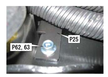
(4) Temporarily install the Intercooler. To install the intercooler, use the Flange Bolt M8 L15 for the side of the Intercooler, and use the Flange Bolt M8 L10 for the lower side.
