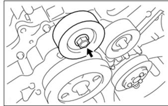
(3) Remove the idler pulley No.2 as shown in the diagram on the right.
