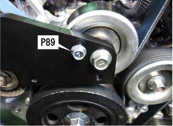
(6) Make sure the belt is placed on all pulleys. Remove the 3mm hexagonal wrench or a similar tool securing the belt. Make sure a proper tension is applied to the belt.
