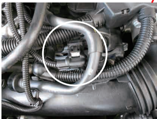
Pressure sensor location (Channel 2)
