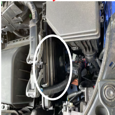
Power Editor installation location
