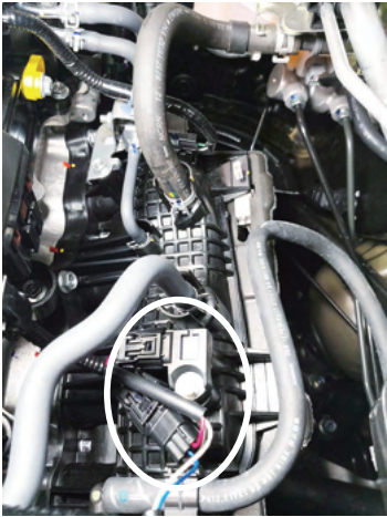
Connect the harness of Power Editor
