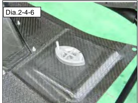
(7) Install the Jack Point Spacer using the provided Flange Nut.
