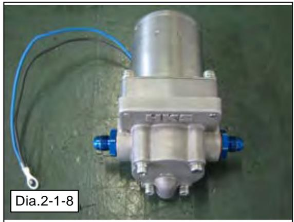
(7) Install the Oil Pump to the bracket using the following provided parts.
