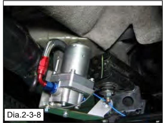
(7) Connect the Hose No.2 to Oil Pump and Core. (Dia.2-3-9)
