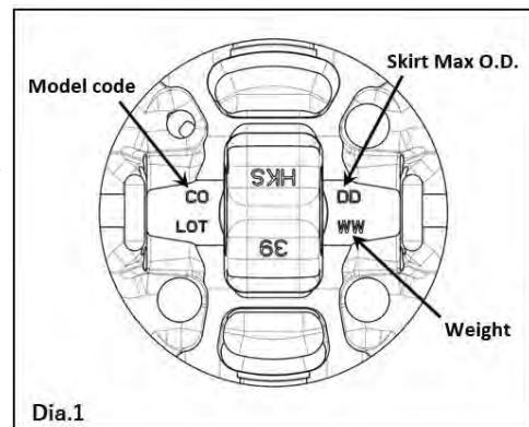
Besides, the HKS piston size is manufactured within 86.455 mm to 86.465 mm.
