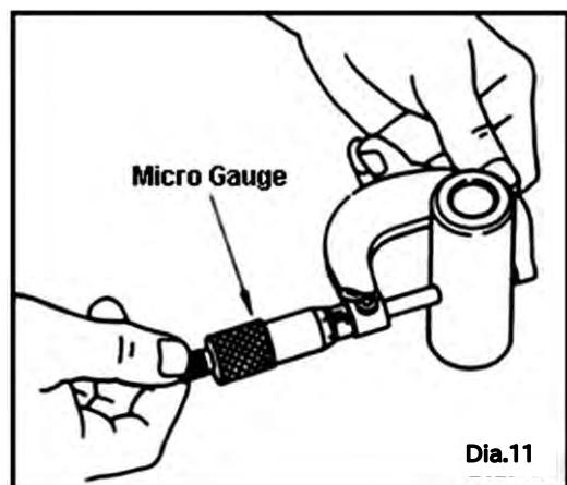
6.3 Calculate the oil clearance of the connecting rod's small end from the O.D. of the piston pin and the I.D. of the connecting rod's small end.
