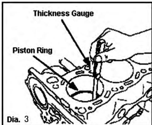
4.2 File off the opening edge with a file or an oil stone to make the clearance within the designated value and C1<C2. (See the table above.)
