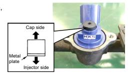
(4)Install the fuel injector cap.
