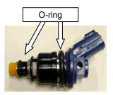
(2)Install the injector to the fuel delivery pipe.
