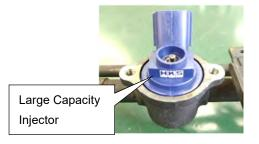
(3)Install the insulator removed in 2. (4) to the injector. At the time, the surface of the insulator with the metal plate faces the injector.
