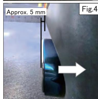
Tighten the bolts and nuts at the flange while pushing the tail to the direction of the arrow.
