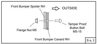
(5) Reinstall the [Front Bumper Spoiler RH] refer to the instruction manual of the body kit TYPE-R.
