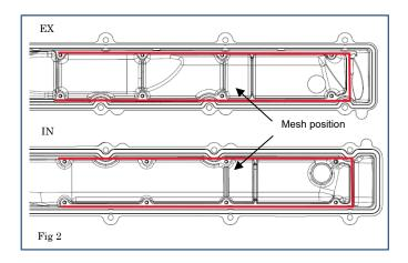
3.4 Assemble the product to the CAM cover with the provided bolt and tighten with the torque of 0.5 kgfm.
