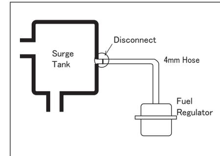
(2) Disconnect the 4mm Hose Between the fuel regulator and surge tank from the surge tank side.
