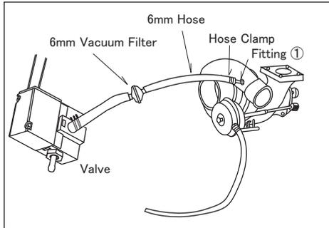
(2) Connect the provided 6mm Hose to fitting ① and the 6mm Vacuum Filter on the NO terminal of the Solenoid Valve.
