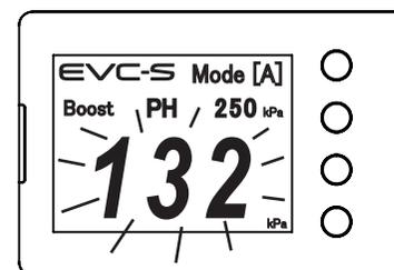
When boost pressure changes from positive pressure to negative pressure, the maximum boost pressure from positive pressure to negative pressure will be displayed blinking for 3 seconds.
