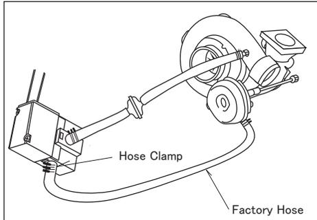
(3) Connect the factory hose from the actuator to the fitting on the COM terminal of the Solenoid Valve.
