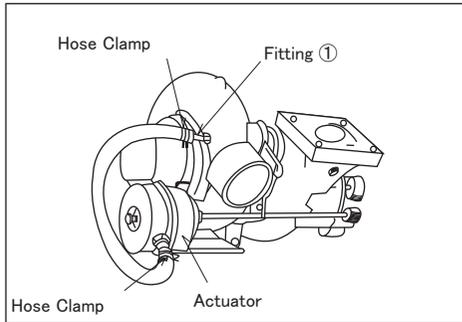
(1) Disconnect the hose connected to the actuator from fitting ① on the compressor side.
