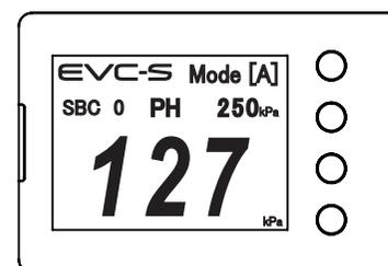
The EVC-S logo will turn red and SBC will be displayed below the logo. While scrambling is in progress, the remaining scrambling time is displayed on the right side of the SBC and a buzzer sounds.
