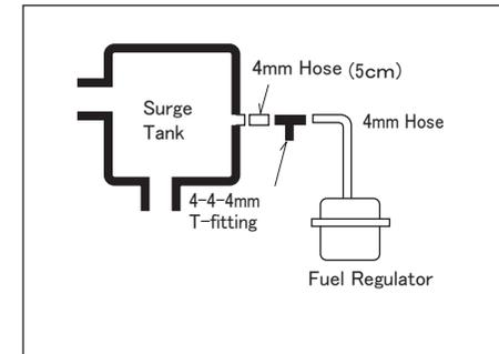
(3) Cut the 4mm Hose to 5cm in length and insert the insert the T-fitting as illustrated in the diagram.
