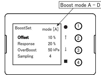
While the main screen is displayed, press and hold button ③ to switch to the boost set screen.
