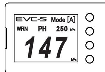
If the boost exceeds the warning setting value and the warning conditions are met, a warning will be activated and the boost will be controlled to be lowered by the set amount. Also, WRN will be displayed flashing under the logo and a buzzer will sound. The warning will be canceled when the boost pressure becomes 5 kPa or less.
