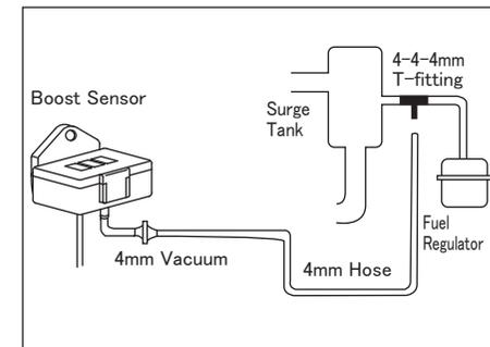
(4) Connect the T-fitting and 4mm Vacuum Filter using the remaining 4mm Hose as illustrated in the diagram.
