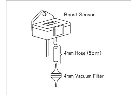
(1) Cut the Hose to 5cm in length and connect the cut hose to the 4mm Vacuum Filter as illustrated in the diagram.
