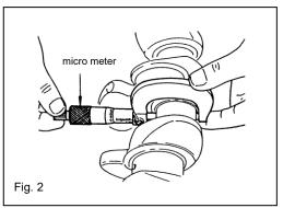
3.4 Calculate the oil clearance by the crank pin diameter checked in 3.3 and the inner diameter of the metal measured in 3.2.
