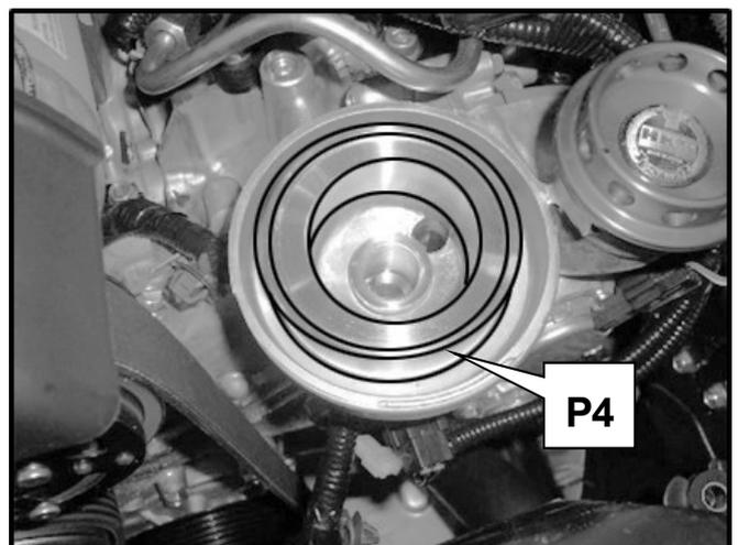
(4) Apply a thin coat of the engine oil to the O-ring.
