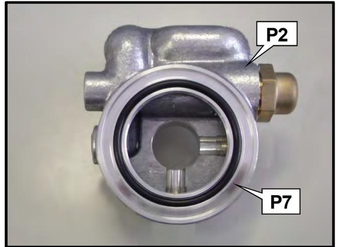
(6) Place the Oil Filter Mount on the Spacer. Temporarily install the mount using the provided Center Bolt.
