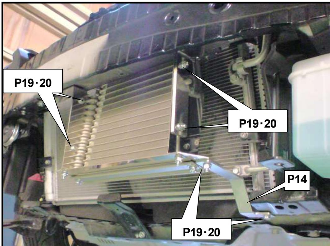
(5) Temporarily install the Core Bracket No.6 to Core Bracket No.4 and the vehicle.
