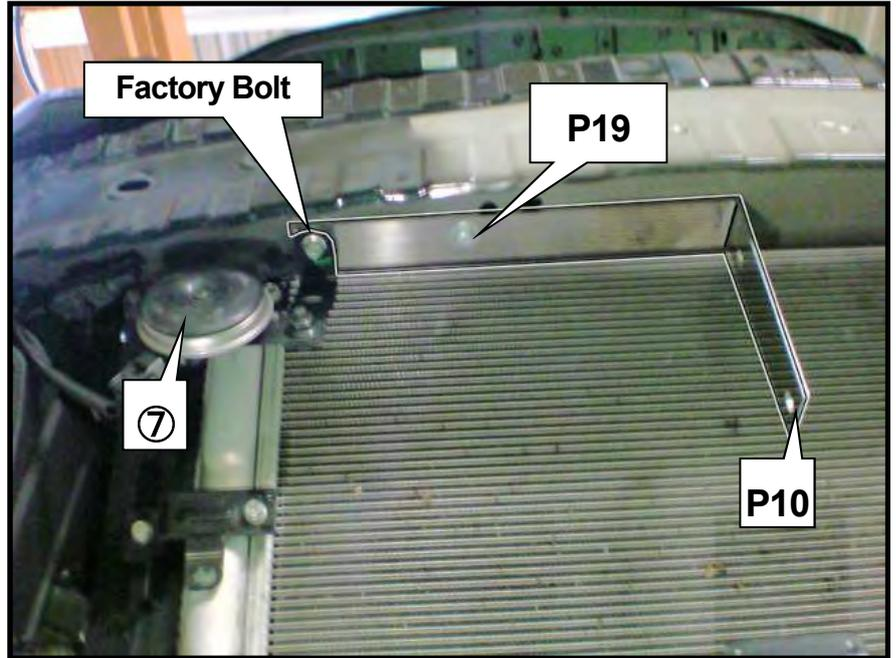
(4) Temporarily install the Oil Cooler Core temporarily assembled in (1) to the Core Bracket No.1 and No.2.
