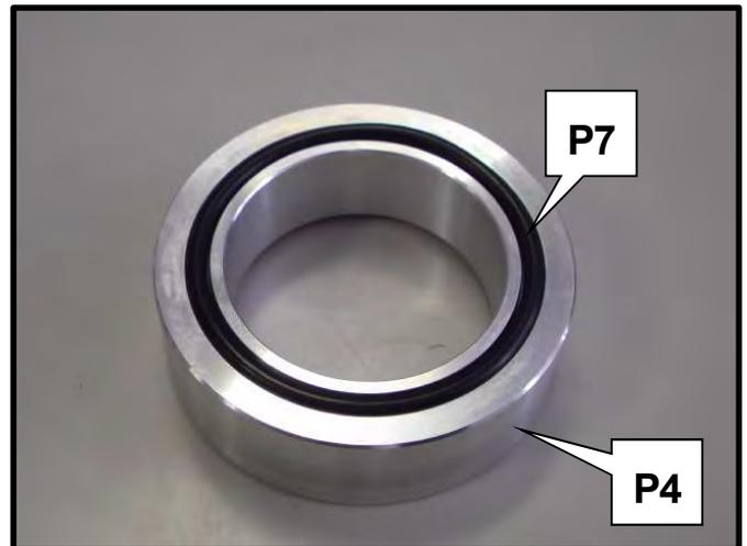
(3) Temporarily install the Spacer with the O-ring to the engine filter installation position.
