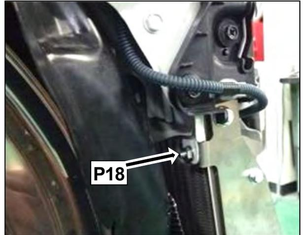
(3) Remove the Oil Cooler Core. Cut off the front fender liner along the mark.
